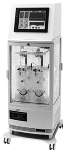
Figure 1 Perfusion preservation machine Machine perfusion system (CMP-X04W; Chuo Seiko, Asahikawa, Japan) was developed in our institute.
